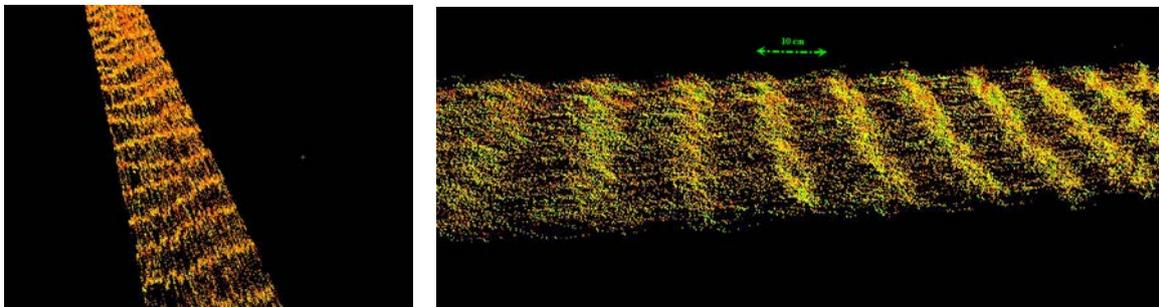
**Figure 4.** High resolution (1mm x 1mm) TLS Scan No.3 revealing the micro-bathymetry of bed ripples under clear shallow water conditions.
