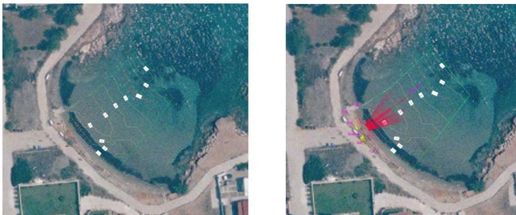
**Figure 2.** Orthophoto of the beach field site with (a) over-imposed bathymetric contours derived from Total station bathymetric survey and (b) with the TLS position and scanned area..
