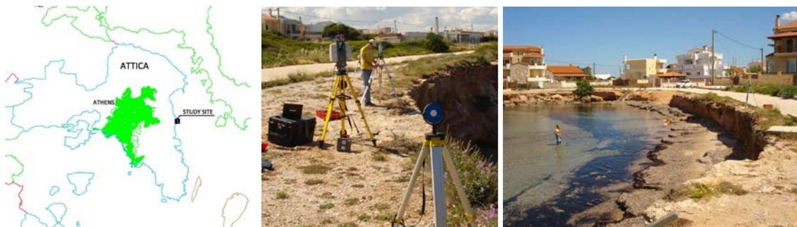
**Figure 1.** a) The study site b) The deployment of the TLS (Terrestrial Laser Scanner), the TS (Total Station) and one of the spherical targets in the field site c) Measuring bathymetry by classical surveying techniques.
