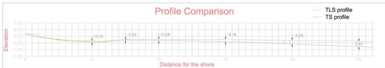
**Figure 5.** A profile comparison derived from Total Station survey (red line) and TLS (green line) measurements.
